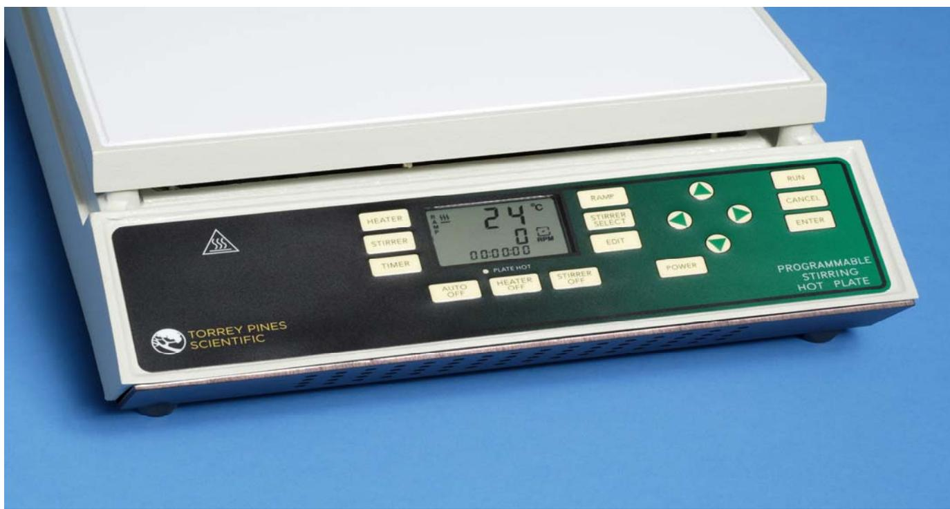
Shown above are the keyboard and display for the HS65 Programmable Digital Hot Plate/Stirrer. This unit has 5-stirring positions and is the most complex unit in the series. Other models in the series will have a single stirring position or no stirrer at all. The keypads will vary depending upon the keys needed for the units in this series with less functions.
