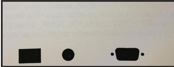
The rear panel shown above has the on/off power switch at the left, the 12 volt dc power input jack in the middle and the RS232 I/O port on the right.
